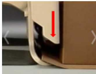
Clamping the slip sheeted load
